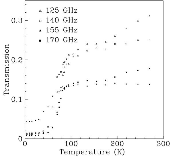
Figure 5: Temperature dependence of the transmission for  $\text{DyBa}_2\text{Cu}_3\text{O}_{7-\delta}$  for 4 different frequencies, illustrating the effect of interference on fixed frequency scans.
