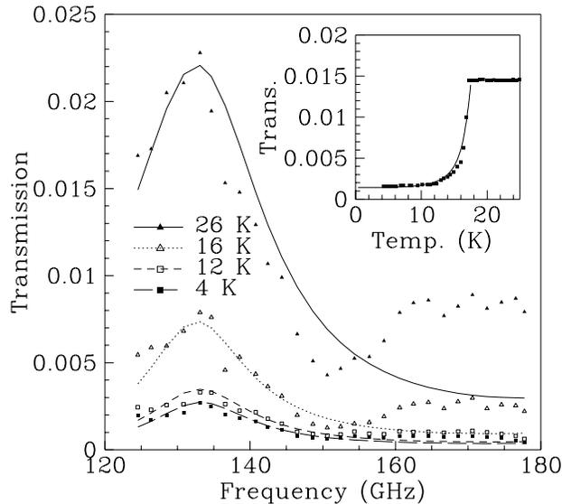
Figure 3: Transmission of NbN on MgO (thickness = 55 nm,  $T_c = 16.5 \text{ K}$ ) for 4 different temperatures (4 K: solid squares, 12 K: open squares, 16 K: open triangles and 26 K: solid triangles) together with their fit. Inset: temperature dependence at 140 GHz together with a BCS-fit using  $\sigma_1(17\text{K}) = 15000 \text{ } \Omega^{-1}\text{cm}^{-1}$  and  $\lambda_L = 400\text{nm}$ .
