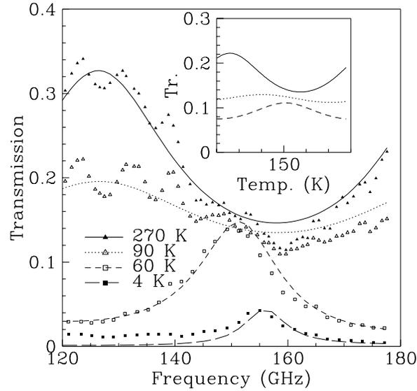
Figure 4: Transmission of  $\text{DyBa}_2\text{Cu}_3\text{O}_{7-\delta}$  on  $\text{LaAlO}_3$  (thickness = 20 nm,  $T_c = 86 \text{ K}$ ) for 4 different temperatures (4 K: solid squares, 60 K: open squares, 90 K: open triangles and 270 K: solid triangles) together with their fit. Inset: Transmission of a thin metallic film for three conductivities. (3000 S/cm: solid line, 5000 S/cm: dotted line, 7000 S/cm: dashed line)
