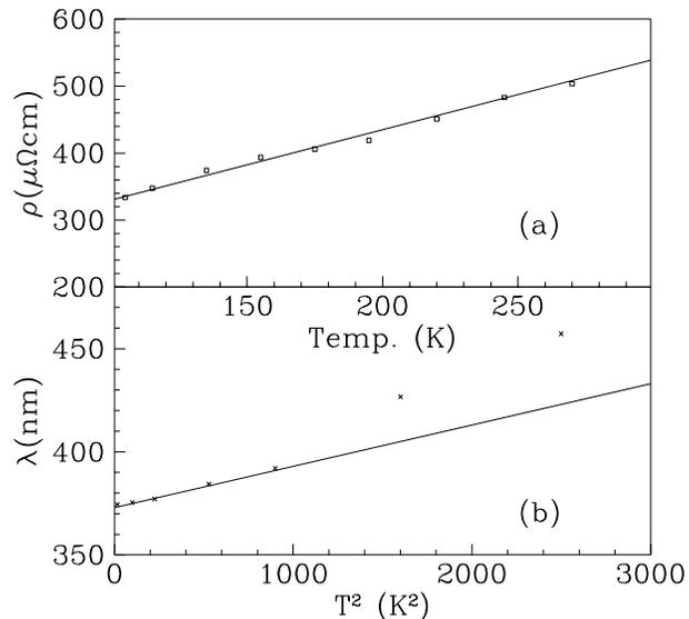
Figure 7: Temperature dependence of the resistivity (a) and the penetration depth (b) for the 20nm thick  $\text{DyBa}_2\text{Cu}_3\text{O}_{7-\delta}$  film.
