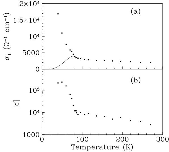
Figure 6: Temperature dependence of the optical conductivity  $\sigma_1$  (a) and  $|\epsilon'|$  (b) for the 20nm thick  $\text{DyBa}_2\text{Cu}_3\text{O}_{7-\delta}$  film. The solid line shows the conductivity of the NbN film, scaled to  $\sigma_1(90\text{K})$ .
