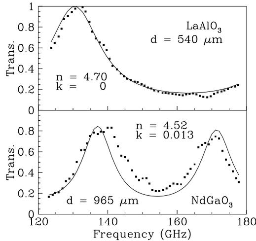
Figure 2: Fabry-Perot resonance spectra for two perovskite substrate materials, LaAlO<sub>3</sub> (top) and NdGaO<sub>3</sub> (bottom).
