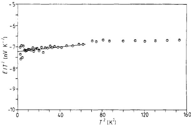
**Figure 5.** Illustration of the phonon drag term in the TEF of the Ag-1.28 at% Pt alloy. The full line is the least-squares fit up to 8 K. The intercept and the slope of the curve give the values  $\frac{1}{2}A$  and  $\frac{1}{4}B$  in equation (1) ( $C = 0$ ), respectively.
