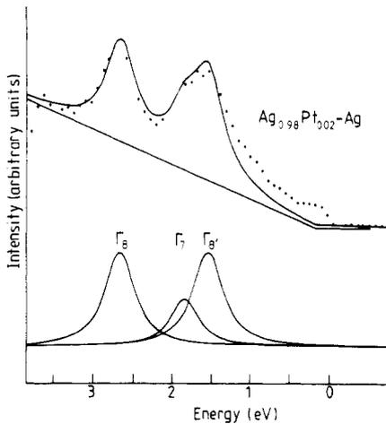
**Figure 4.** Comparison of the experimental (dots) 1.90 at% alloy data with the theoretically simulated spectrum (full curve). Also shown are the separate contributions of the three irreducible representations. The parameters used are  $\zeta = 0.39$  eV,  $10Dq = 0.43$  eV and  $\text{FWHM} = 0.45$  eV.
