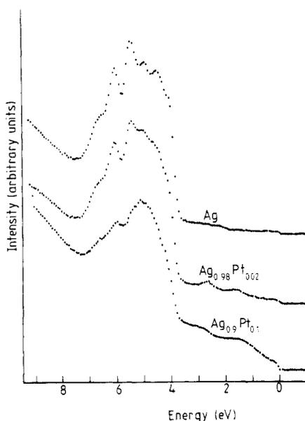
**Figure 1.** UPS valence band spectra of pure Ag and the Ag-1.90 at% Pt and Ag-10 at% Pt alloys.
