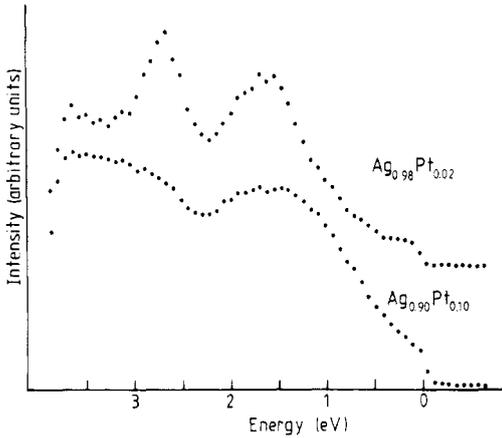
**Figure 2.** Difference spectra (alloy – pure Ag) for the Ag–1.90 at% Pt and Ag–10 at% Pt alloys.
