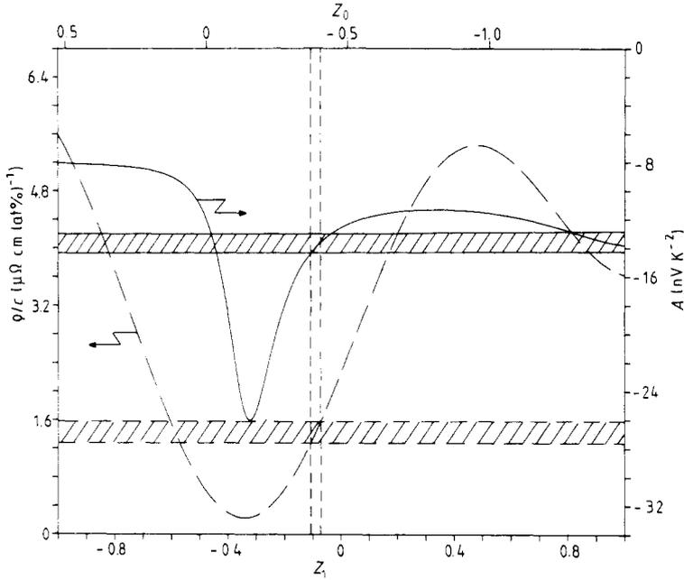
**Figure 6.** Resistivity ( $\rho/c$ ) (broken curve) and TEP coefficient ( $A$ ) (full curve) as functions of the partial screening charges  $Z_0$  and  $Z_1$ . The values consistent with the experimental data lie within the shaded areas. The Friedel sum is  $\Delta Z = -0.85$ . The vbs parameters adopted from the UPS spectra are  $E_{3/2} = -2.65$  eV,  $E_{5/2} = -1.6$  eV and  $2\Delta = 0.45$  eV.
